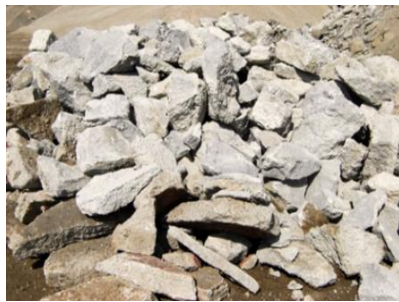
Step 1. Demolished concrete collection
