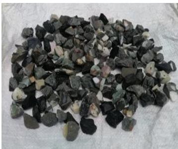
Step 5. Washed stone with distilled water
