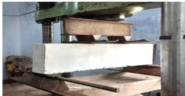
Fig. 6. Four point bending test of beam
