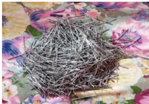
Fig. 2. 30 mm steel fiber
