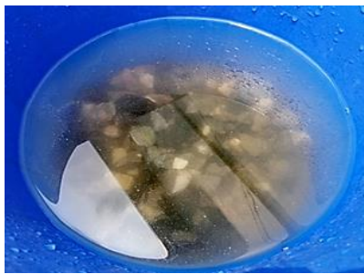
Step 4. Soaking of stone in 0.1 M HCl solution
