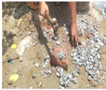
Step 2. Manual crushing
