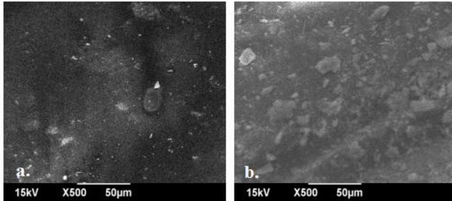
Fig. 1. a). SEM micrograph of  $\beta$ -cyclodextrin, b). SEM micrograph of *Citrus limonium*- $\beta$ -cyclodextrin composite
