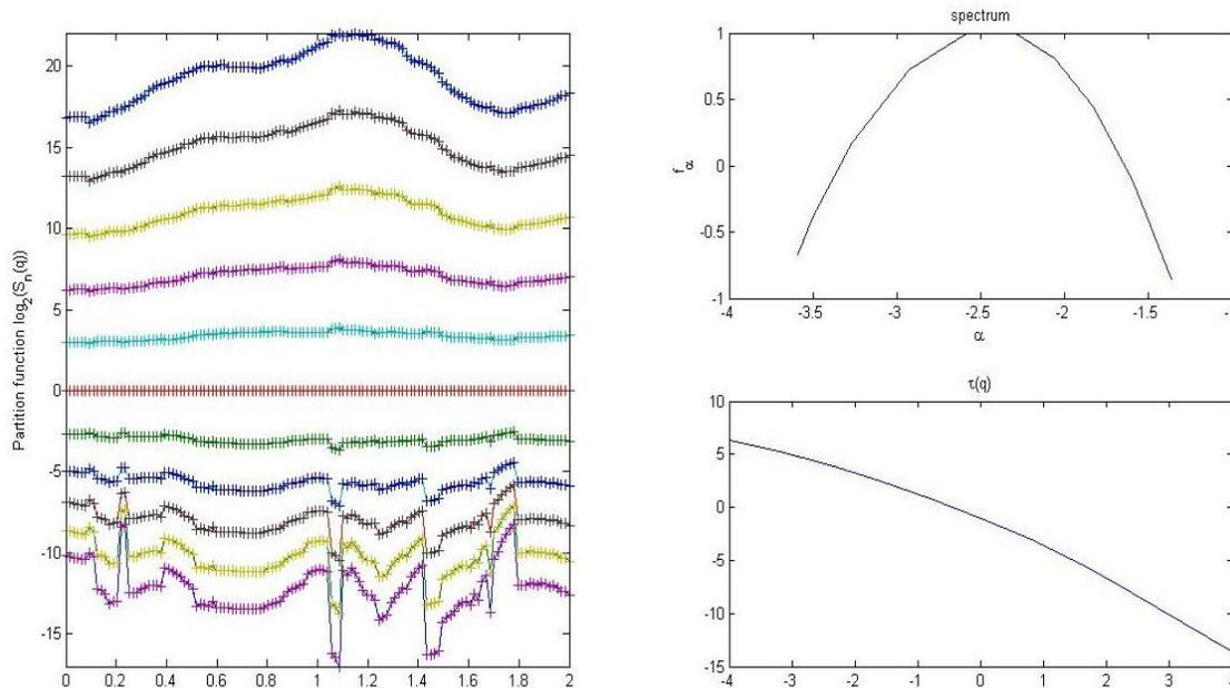
**Fig. 5. Multifractal analysis of Solar Cycle 23 using CWT (Morlet wavelet of size 8 and 128 voices, LS regression and local maxima). In figure Left panel show the Legendre spectra and Right (upper) panel gives the singularity spectrum and Right (lower) panel for scaling function of the considered time series**
