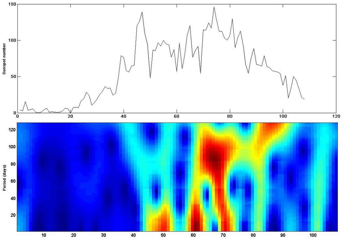
**Fig. 8. CWT of Solar Cycle 24 using a Morlet Wavelet of size 8 and 128 voices. In figure X axis represents the number of samples and Y axis represents scale. The upper panel shows the raw data of the time series and lower panel its continuous wavelet transform (CWT)**
