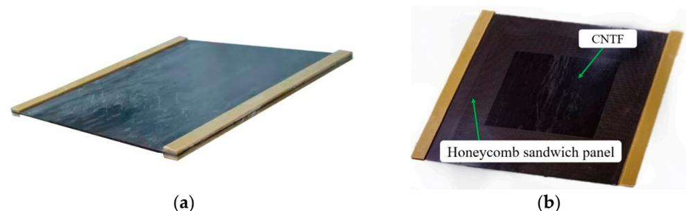
Figure 5. Specimens after curing: (a) unprotected specimen; (b) protected specimen.
